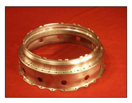
However, the following is the diffuser case design for the 757 jet engines and it is quite different from that shown at the Pentagon. That is due to the difference between "dual-chamber turbojet" versus the newer "high bypass jet fan" designs found on the 757 and 767 jet airplanes.
